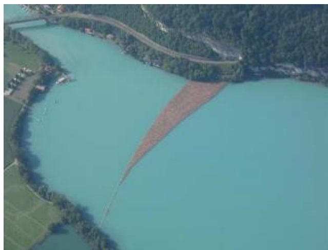
Figure 33: Large wood barriers on Lake Brienz during the 2005 flood event (Photo: Federal Office for the Environment, Switzerland).
