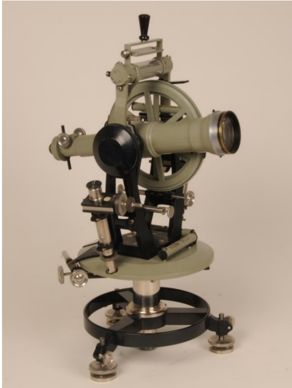
Abb. 12: Theodolit Kern, 1913 (swisstopo)
