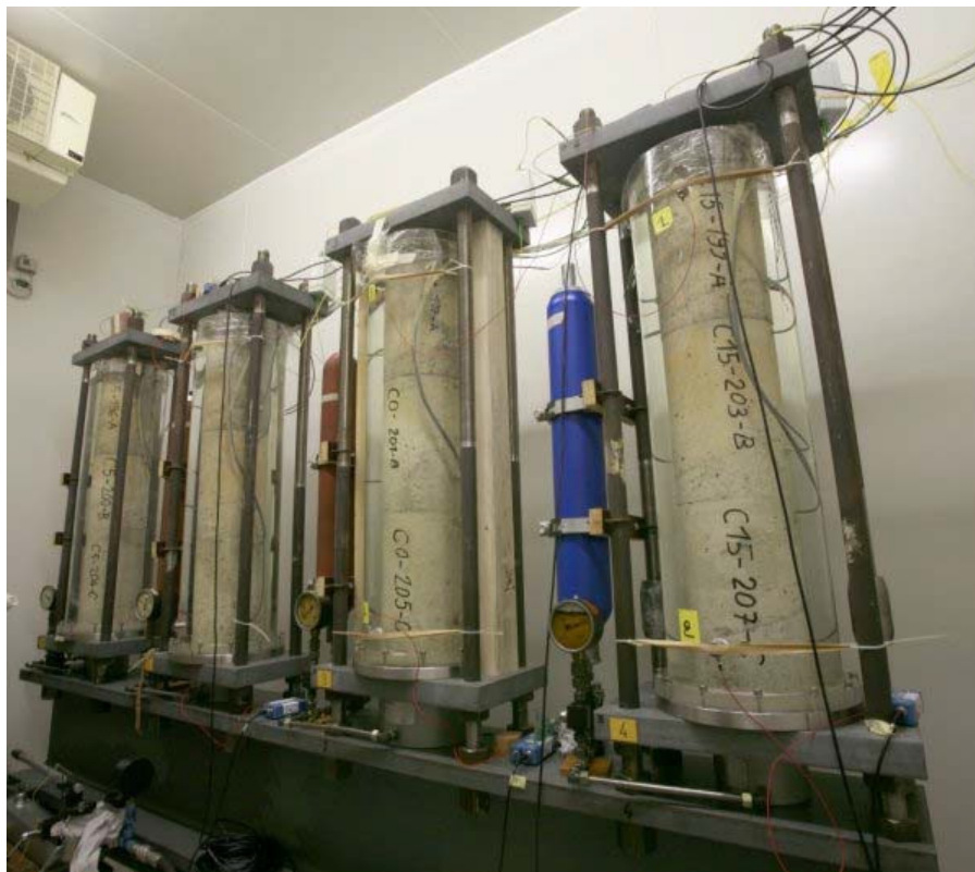
Figure 6. Set up for tests under uniaxial compression. The Perspex jackets allow the samples to be maintained immersed in sodium hydroxide solution to avoid leaching
