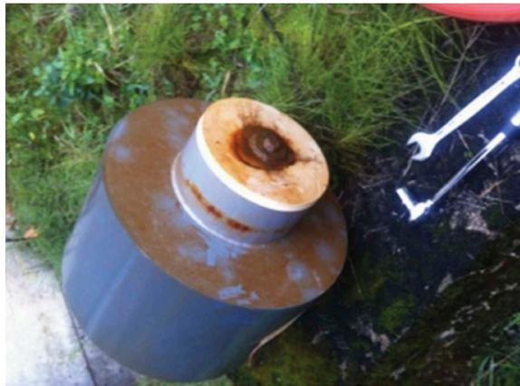
Figure 8. Corroded float stem.
