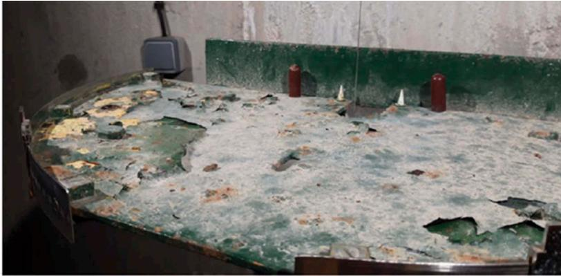
Figure 7. Pendulum table achieved electrolysis.
