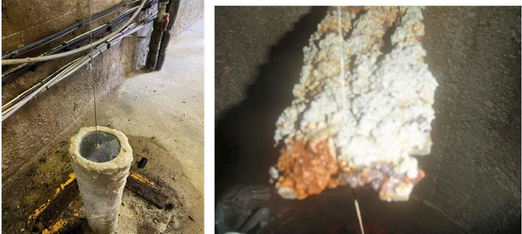
Figure 5. Examples of calcite on pendulum components.
