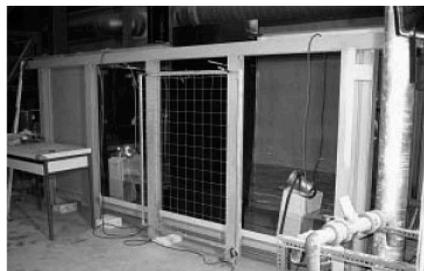
Figure 3. Photograph of experimental tank, including thrusters.
