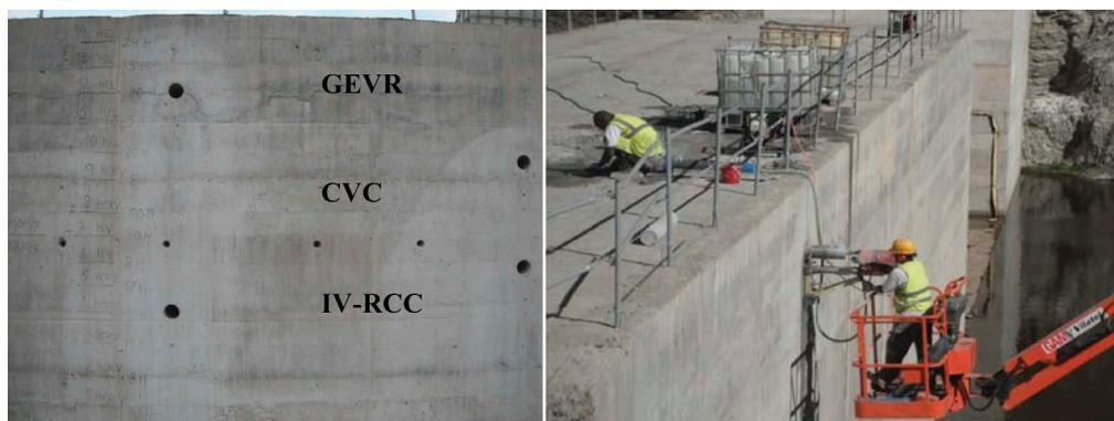
Figure 3. Evaluation of IV-RCC vs. CVC and GEVR facing systems through drilled cores.
