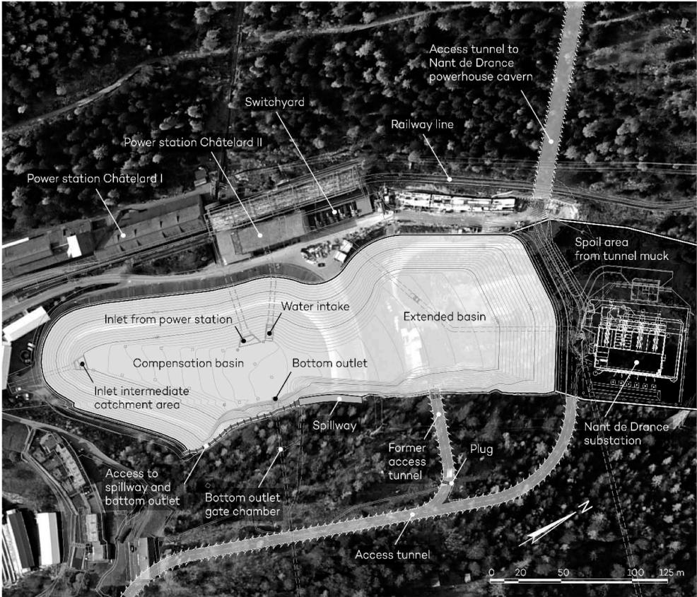
Figure 1. Châtelard compensation basin - original part (left side) and enlarged part (right side).
