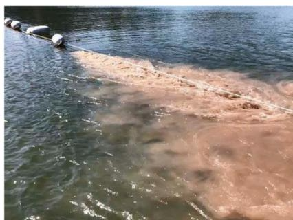
Figure 7. Discharge of sediments from the ejector dredge during SAT.
