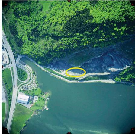
Figure 8. The Zingel quarry. The marked part of the early excavation was to be filled with waste slag, while siliceous limestone is still being mined in the rear part (Lumpert ZKRI, 2000).
