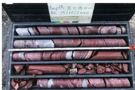
Figure 6. Typical core box sample representation from borings near Hydropower Koman. [A.L.T.E.A. & Geostudio 2000].
