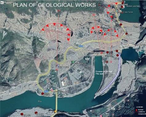
Figure 3. Plan of geological works identifying landslide area [A.L.T.E.A. & Geostudio 2000].
