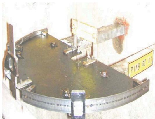
Figure 12. Pendulum equipped with a vertical measuring device.
