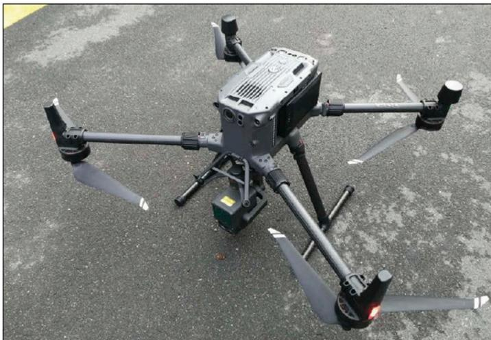
Figure 4. Drone for monitoring of dams.
