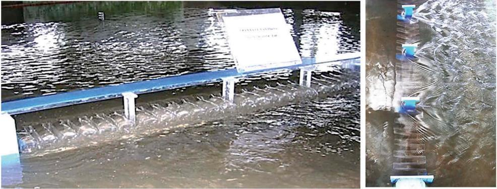
Figure 8. a) and b) Hydraulic model tests for submerged flows.
