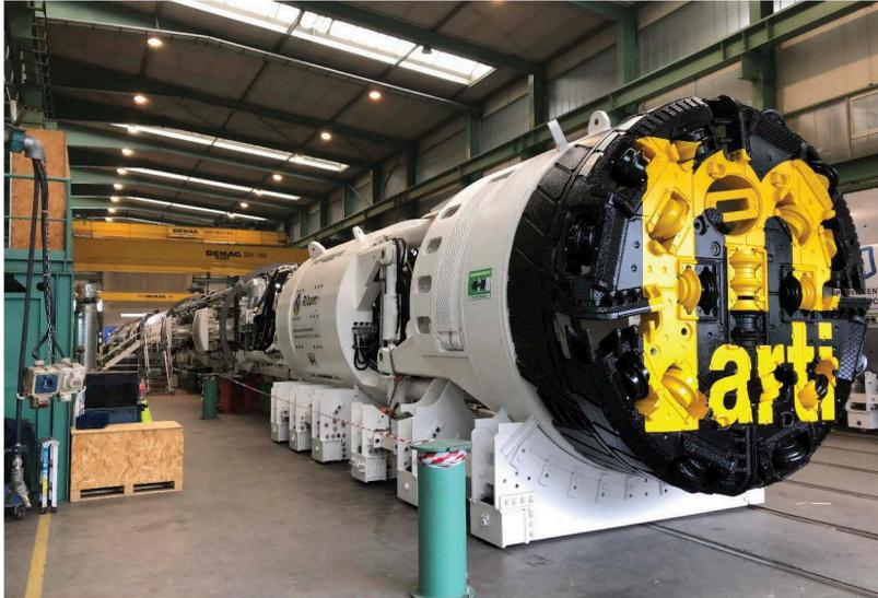
Figure 4. Pre-assembled TBM at the Herrenknecht factory.
