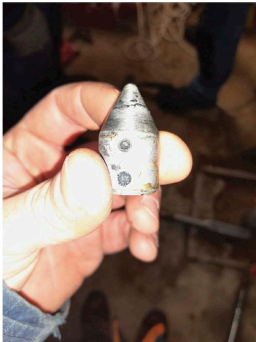
Figure 3. Cable clamp with corroded screws.
