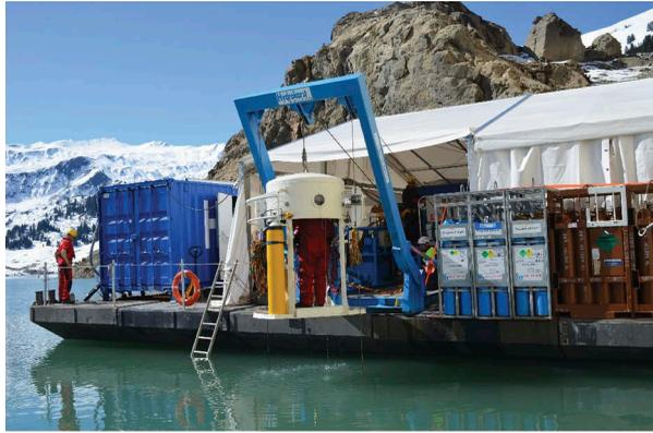
Figure 10. Pontoon fully equipped for wet bell diving.
