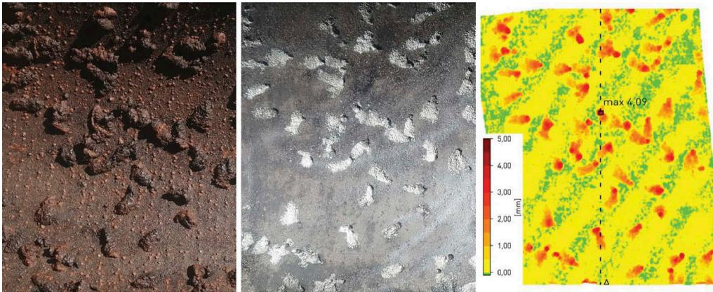
Figure 7. (a) and (b) Heavily corroded inner pipe surface before and after cleaning; (c) Representation of the results of the surface measurement with laser scan © Kager.
