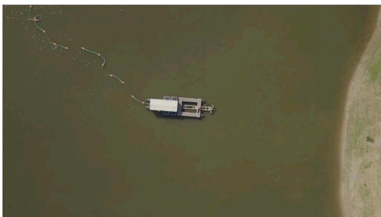
Figure 2. SediMover with visible cable connection to anchor points.
