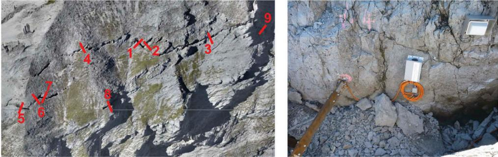
Figure 3. Aerial photograph of the Schafselbsanft cliff with the nine cracks that are monitored with crackmeters (left). Example of the installation on site with a crackmeter, the data logger and a transmission unit (right).
