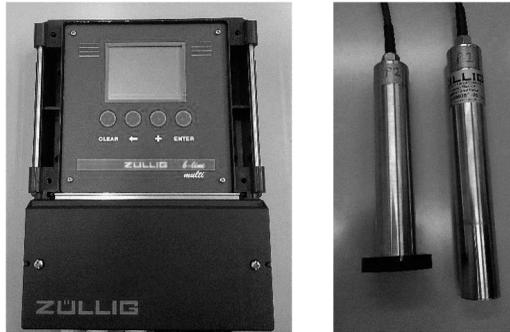
Figure 6. Züllig Transmitter (left) and COSMOS-25 Turbidity Probes (right).
