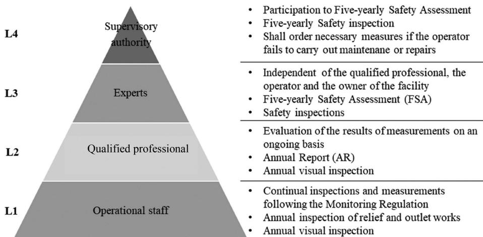
Figure 1. The four levels and their main tasks (non-exhaustive) according to WRFA and WRFO.
