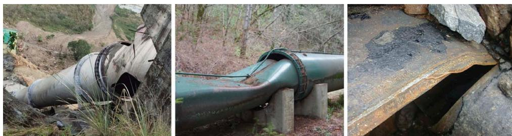
Figure 1. (a) Failure of a penstock due to material defect © www.icnnational.com; (b) Failure of a penstock due to pressure surge © www.fateclub.org; (c) Crack caused by ice formation inside © Kager.
