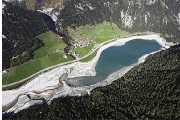
Figure 1. Sedimentation of Sufers reservoir, Grisons, Switzerland (Amini et al., 2020).
