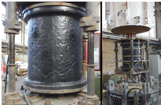
Figure 4. Left: Sample ready for testing inside the membrane Right: Sample before closing the apparatus (KIT 2021).
