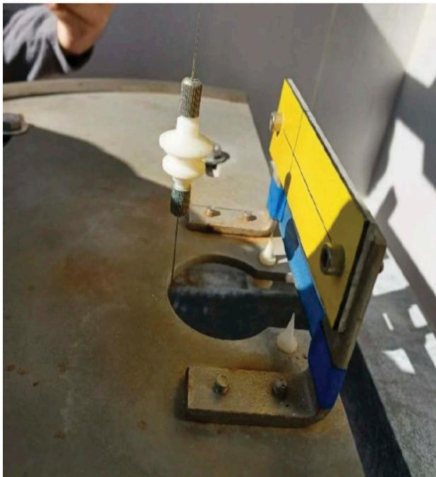
Figure 10. Pendulum wire touching the table during a heat wave.
