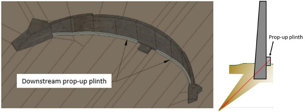
Figure 3. Downstream prop-up plinth: perspective illustration view (left) and typical cross section (right).
