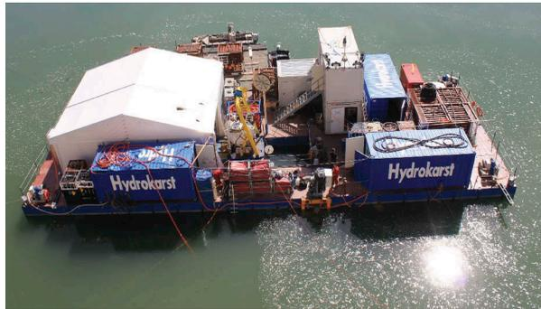
Figure 11. Pontoon equipped for bell diving in saturation.
