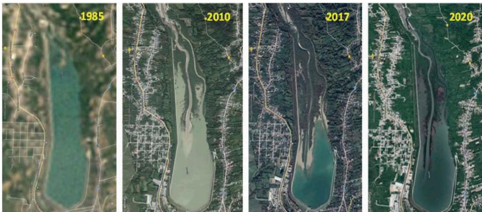
Figure 8. The evolution of the silting of Pucioasa reservoir between 1985 and 2020.
