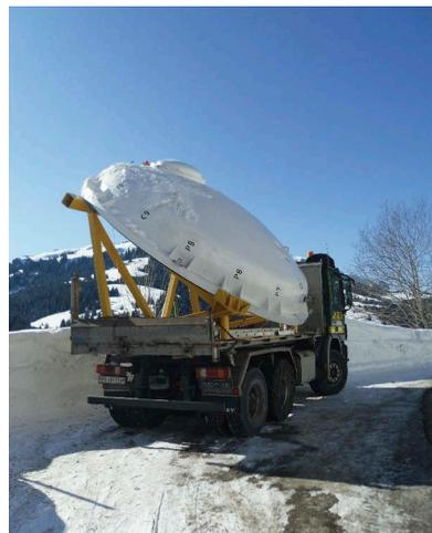
Figure 13. Right: Truck transporting the obturator on a special frame towards Hongrin dam (Switzerland).
