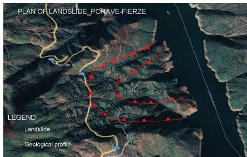
Figure 8. Landslide view at Porava area, Fierza dam. [A.L.T.E.A. & Geostudio 2000].
