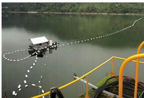
Figure 6. The floating ejector dredge operating in Necaxa Reservoir in 2022.
