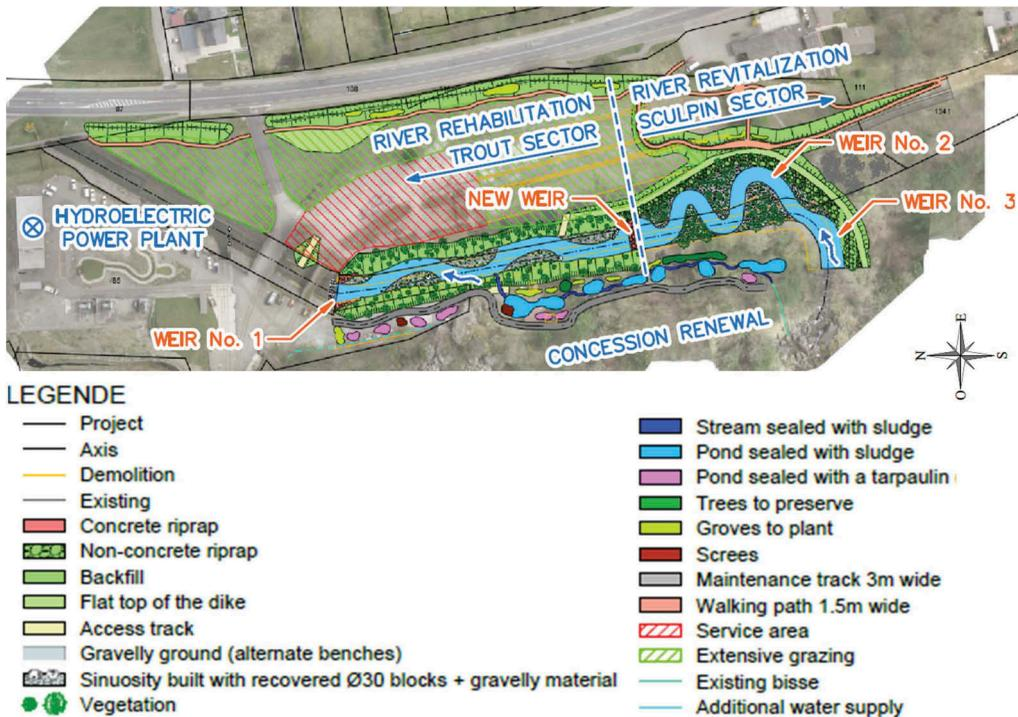
Figure 3. Overall view of the revitalization project on the upstream sector of the Salanfe in the plain.
