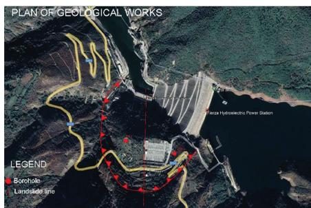
Figure 7. Gropaj landslide view at Fierza dam. [A.L.T.E.A. & Geostudio 2000].
