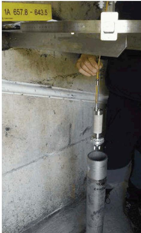
Figure 9. Controlling the free domain of a pendulum.
