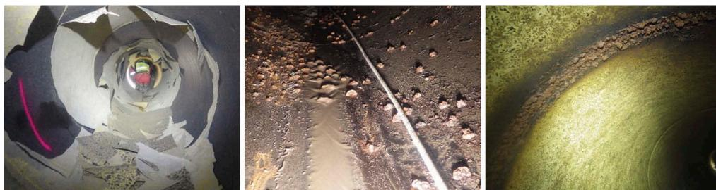
Figure 3. (a) Peeling of the coating due to inadequate surface roughness; (b) Punctual damage; (c) Absence of the coating on site-produced welds © Kager.
