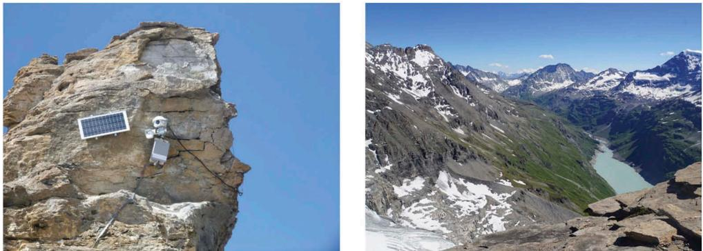
Figure 2. System installed on a rock pillar with the housing containing the camera, a solar panel and a control cabinet (left). View on the Mauvoisin reservoir and on the Gietro glacier (bottom right corner of the right panel).
