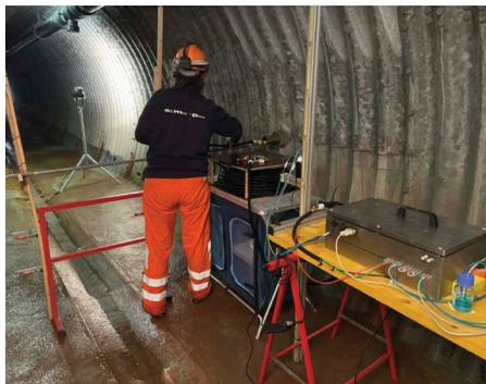
Figure 9. Deformation measurement of the landfill base in the Zingel landfill with GRIMONIT. A sliding rod is used to place the probe into the inclinometer tubes in meter increments. The pressure signal is transmitted via the 50 m long pipe drum. The differential pressure between the probe in the inclinometer tube and the moving reference probe is used to calculate the course of the inclinometer tube.
